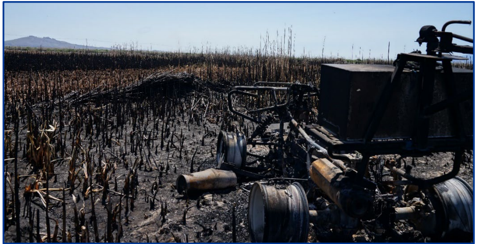
The burned ATV location in relation to the impacted tule berm. The ATV operator’s escape path and safety zone is located 15 feet to the left of the ATV.
